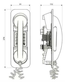
dimensions mm (W x H x D) 91,0 x 278,0 x 110,0 weight 700 g
