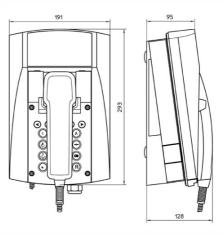
dimensions (W x H x D) 191,0 x 293,0 x 128,0 mm weight 2,3 kg
