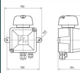
dimensions (W x H x D) 150,0 x 190,0 x 104,0 mm weight 1,5 kg
