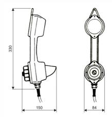
dimensions (W x H x D) 84,0 x 330,0 x 150,0 mm weight 1,4 kg
