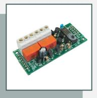
Plug in card with 2 relays (e.g. for opening doors, switching lights, etc.) controlled by a remote telephone set or by the same SANIVOX (code 7133630) through specific programmable secret code; output on one switch over contact for each relay, with power rating (on resistive charge) 250mA/24Vdc or 500mA/230Vac; possibility of activating automatically one relay when a call starts till to the automatic hanging up of the same (for switching-on external signals, cameras or other devices).
