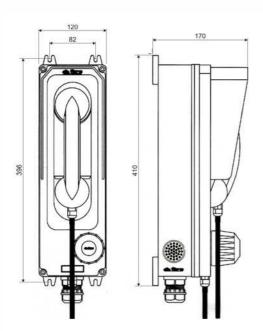
dimensions mm (W x H x D) 120,0 x 380,0 x 170,0 weight 2,95 kg
