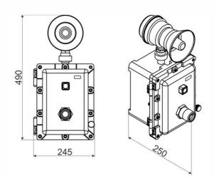
dimensions (W x H x D) 245,0 x 490,0 x 250,0 mm weight 12,6 kg
