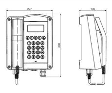
dimensions (W x H x D) 227,0 x 293,0 x 135,0 mm weight 6,28 kg
