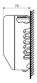
dimensions mm (W x H x D) 106,0 x 140,0 x 73,0 weight 500 g
