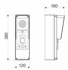
dimensions (W x H x D) 120,0 x 380,0 x 170,0 mm weight 1,5 kg
