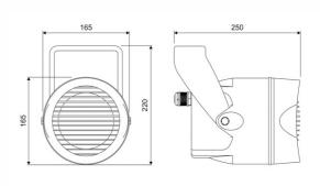
dimensions (W x H x D) 165,0 x 220,0 x 250,0 mm weight 1,85 kg
