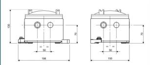
dimensions (W x H x D) 198,0 x 150,0 x 130,0 mm weight 3,0 kg
