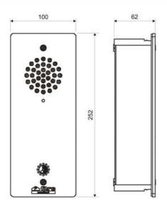
dimensions mm (W x H x D) 100,0 x 252,0 x 64,0 weight 930 g
