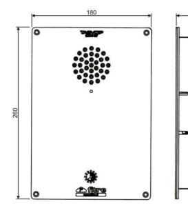
dimensions mm (W x H x D) 180,0 x 260,0 x 57,0 weight 1,45 kg
