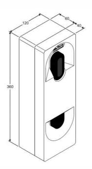
dimensions mm (W x H x D) 120,0 x 360,0 x 100,0 weight 4,0 kg
