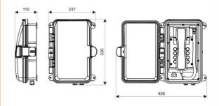
dimensions (W x H x D) 237,0 x 330,0 x 110,0 mm weight 2,3 kg
