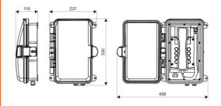
dimensions (W x H x D) 237,0 x 330,0 x 110,0 mm weight 2,3 kg
