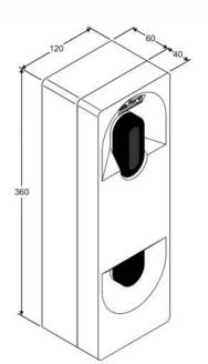
dimensions mm (W x H x D) 120,0 x 360,0 x 100,0 weight 4,0 kg
