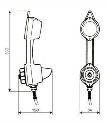
dimensions (W x H x D) 84,0 x 330,0 x 150,0 mm weight 1,4 kg
