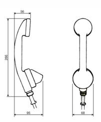
dimensions (W x H x D)  $58.0 \times 266.0 \times 95.0 \text{ mm}$  weight 700 g
