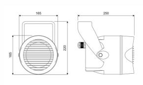
dimensions (W x H x D) 165,0 x 220,0 x 250,0 mm weight 1,85 kg
