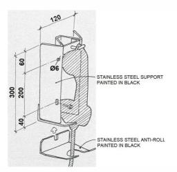
dimensions (W x H x D) 120,0 x 300,0 x 110,0 mm weight 1,0 kg
