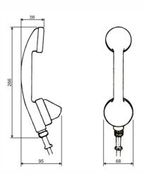
dimensions (W x H x D)  $58.0 \times 266.0 \times 95.0 \text{ mm}$  weight 600 g
