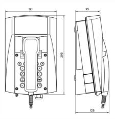
dimensions (W x H x D) 191,0 x 293,0 x 128,0 mm weight 1,7 kg
