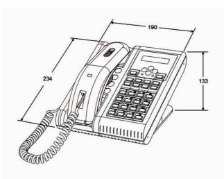
dimensions mm (W x H x D) 190,0 x 133,0 x 234,0 weight 1,75 kg
