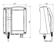
dimensions (W x H x D) 227,0 x 293,0 x 135,0 mm weight 5,21 kg
