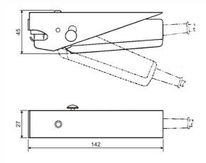
dimensions (W x H x D)  $27,0 \times 142,0 \times 45,0 \text{ mm}$  weight 400 g
