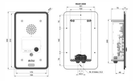
dimensions mm (W x H x D) 195,0 x 330,0 x 81,0 weight 1,97 kg
